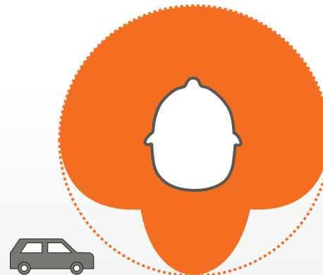
Figure 3. Illustration of how null directions can attenuate localised, dominant noise sources. Thanks to the spatially informed noise estimate, the depth of a null direction is stronger for sounds placed further towards the back.
